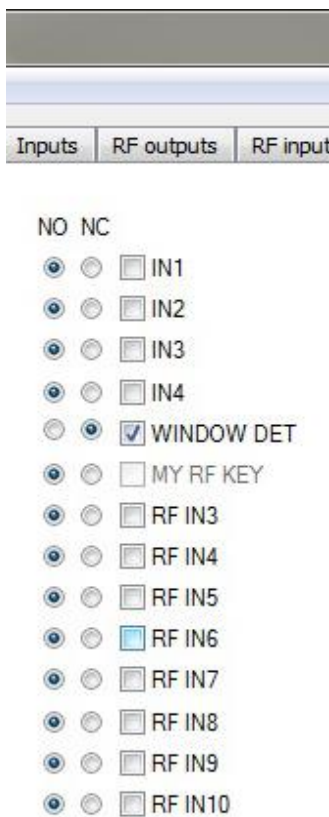
Image 30: Tab "ARM/DISARM" – selection of inputs of the guarded zone and their standby mode.
